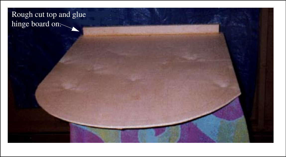
Figure 12 Attaching hinge board
